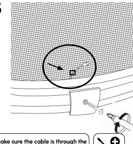
Thread the cable through the highlighted hole in the mesh and slide up the clip over the ridge of the bottom of the back mesh
