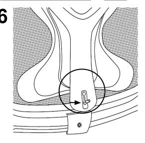
To install the posturefit module, slide the bracket over the rails and push down on each side. Ensure the cable is reachable from behind the pad
